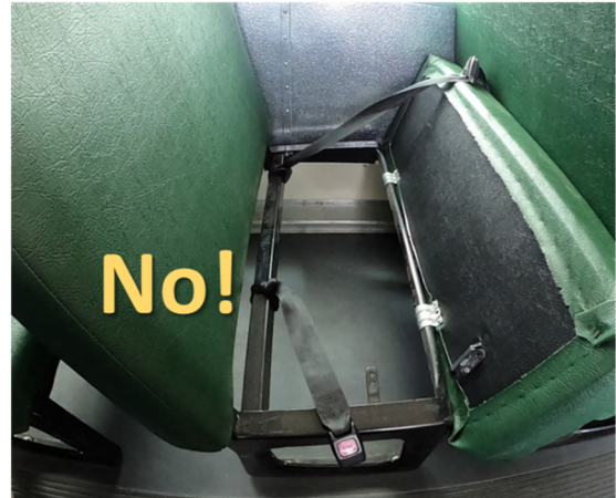
Seat belt knotted around the bus frame
